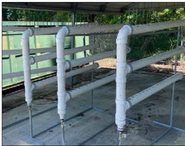
Pictured: Typical motor oil bottle drain racks
