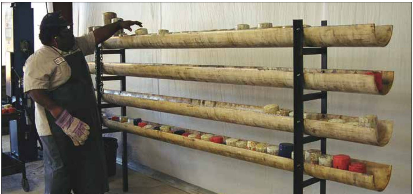
Pictured: A motor oil filter drain rack
